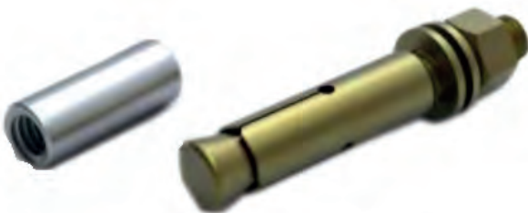
Extension and Anchor Bolt 1/4" to 5/8" Ø21 X 55 mm - Extension 1/4" to 5/8" Ø21 X 122 mm Material: Steel Galvanized or bichromatic finish
