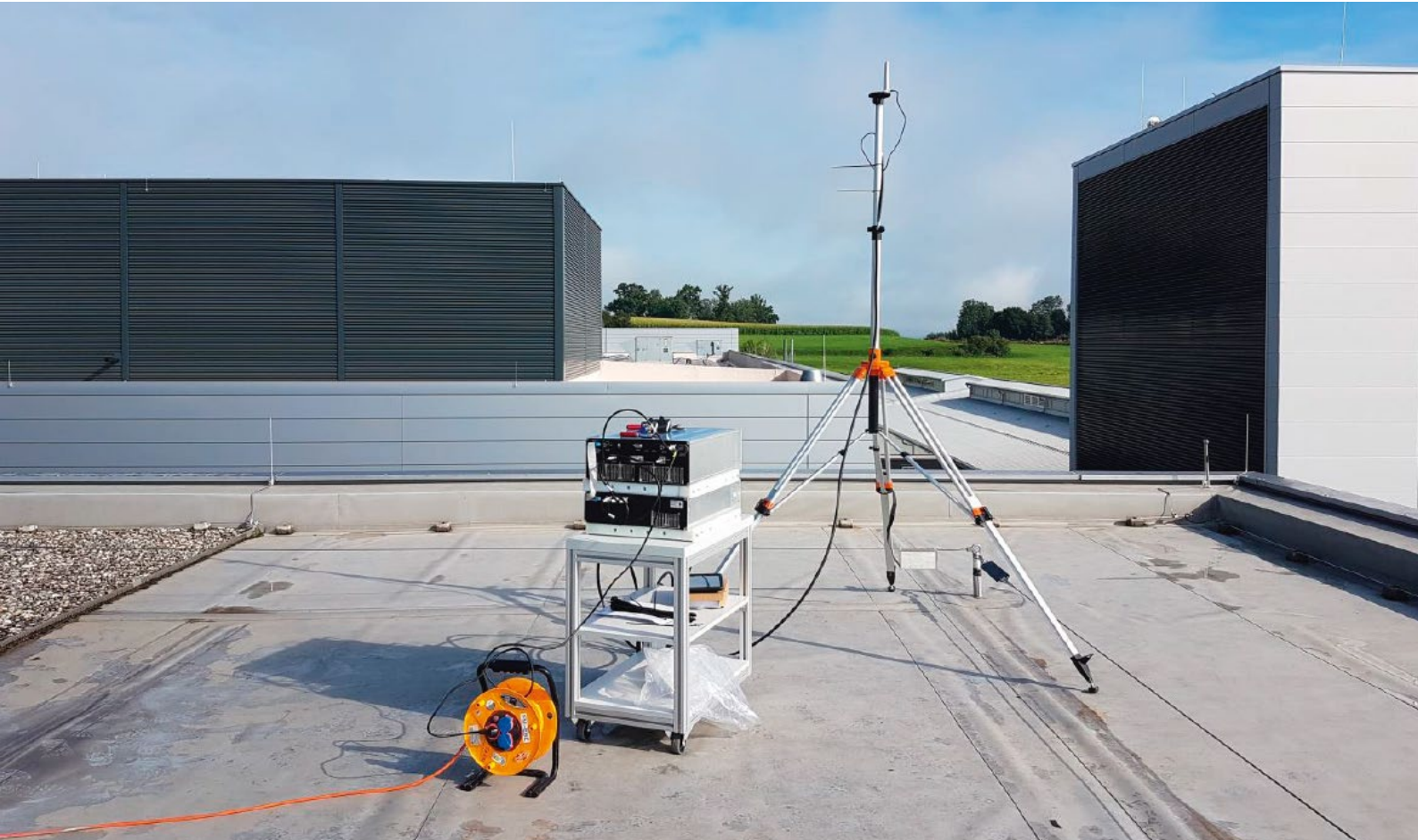
Test setup of transmitter location
